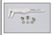
The RAPCO PN. RA-VAC MEASURE KIT is an inspection kit used to help determine when a dry air pump should be replaced. The kit comes with a caliper to measure vane wear, along with three extra cap screws and three extra lock washers, which are used to seal the inspection port found on all new RAPCO dry air pumps. This kit is designed to be used in compliance with RASL-006 or in the event one should lose the cap screw and/or lock washer during an inspection.
